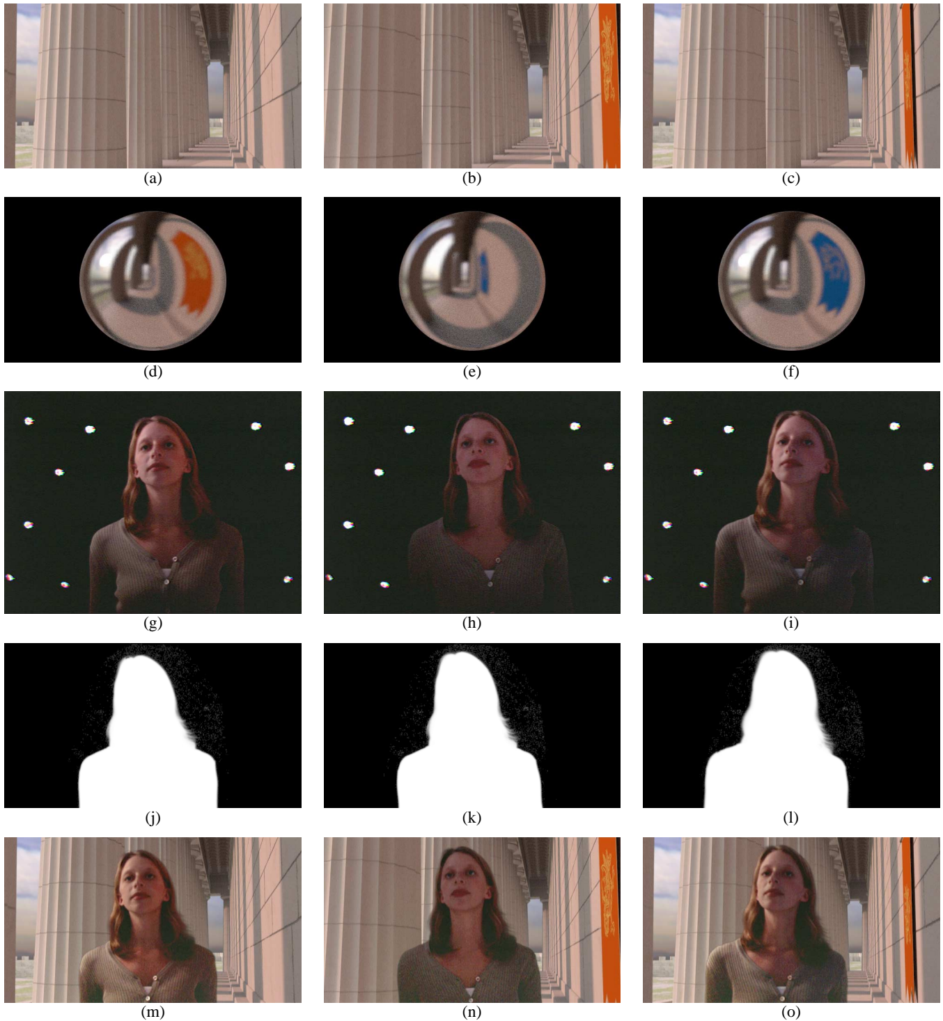
Figure 13: Moving Sequence Results (a-c) Three frames of an animated background plate, rendered using the Arnold global illumination system. The camera moves backwards down the collonade of the Parthenon illuminated by late afternoon sun. (d-f) The corresponding light probe images formed by rendering an orthographic view of a reflective sphere placed where the actor will be in the scene. The sphere goes into and out of shadow and reflects the red and blue banners on the right wall of the gallery. (g-i) The corresponding frames of the actor from the live-action shoot, illuminated by the lighting in (d-f), before brightness falloff correction. (j-l) The processed mattes obtained from the infrared compositing system, with the background in black (m-o) The final composite of the actor into the background plates after brightness falloff correction. The actor begins near the red banner, moves into the shadow of a column, and emerges into sunlight near the blue banner. (The blue banner appears directly to the right in the lighting environment (f) but has not yet entered the field of view of the background plate in (c) and (o).) Comparing (m) to (o), it can be seen that the shadowed half of the actor's face receives subtle indirect illumination from the red and blue banners.
