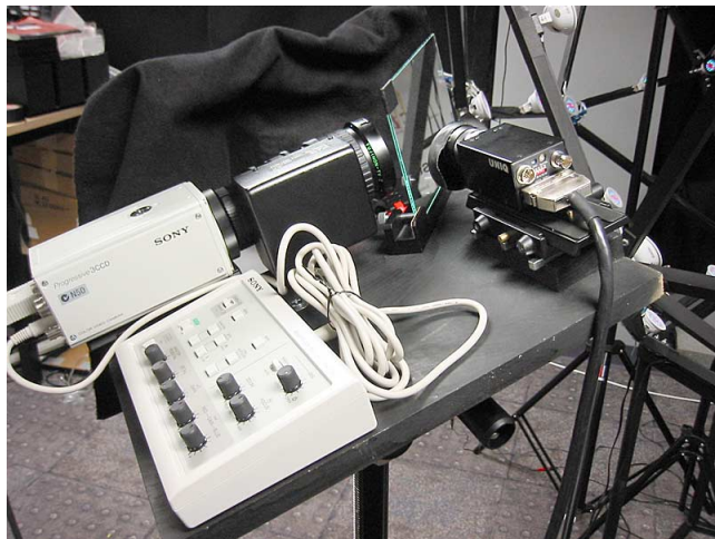
Figure 4: The Camera System The camera system consists of a 3-CCD Sony DXC-9000 color video camera to record the actor (left) and a Uniq Vision UP-610 monochrome video camera to record the infrared matte. The cameras are placed with coincident nodal points using a 30R / 70T beam splitter.
