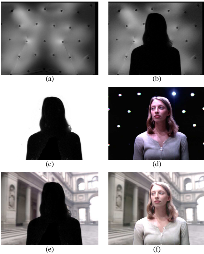
Figure 6: The Matting Process (a) The cloth backing, illuminated by the six infrared light sources. The dark circular disks are the fronts of the RGB lights appearing through holes in the cloth. (b) An infrared image of the actor in the light stage. (c) The matte obtained by dividing image (b) by the clean plate in (a); the actor remains black and the background divides out to white. (d) The color image of the actor in a lighting environment. (e) A corresponding environment background image, multiplied by the matte in (c) leaving room for the actor. (f) A composite image formed by compositing (d) onto (e) using the matte (c). The actor's image has been adjusted for color balance and brightness falloff as described in Section 4.
