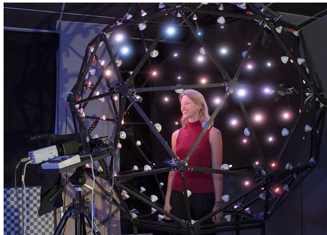
Figure 1: Light Stage 3 focuses 156 red-green-blue LED lights toward an actor, who is filmed simultaneously with a color camera and an infrared matting system. The device composites an actor into a background environment as illuminated by a reproduction of the light from that environment, yielding a composite with consistent illumination. In this image the actor is illuminated by light recorded in San Francisco's Grace Cathedral.
