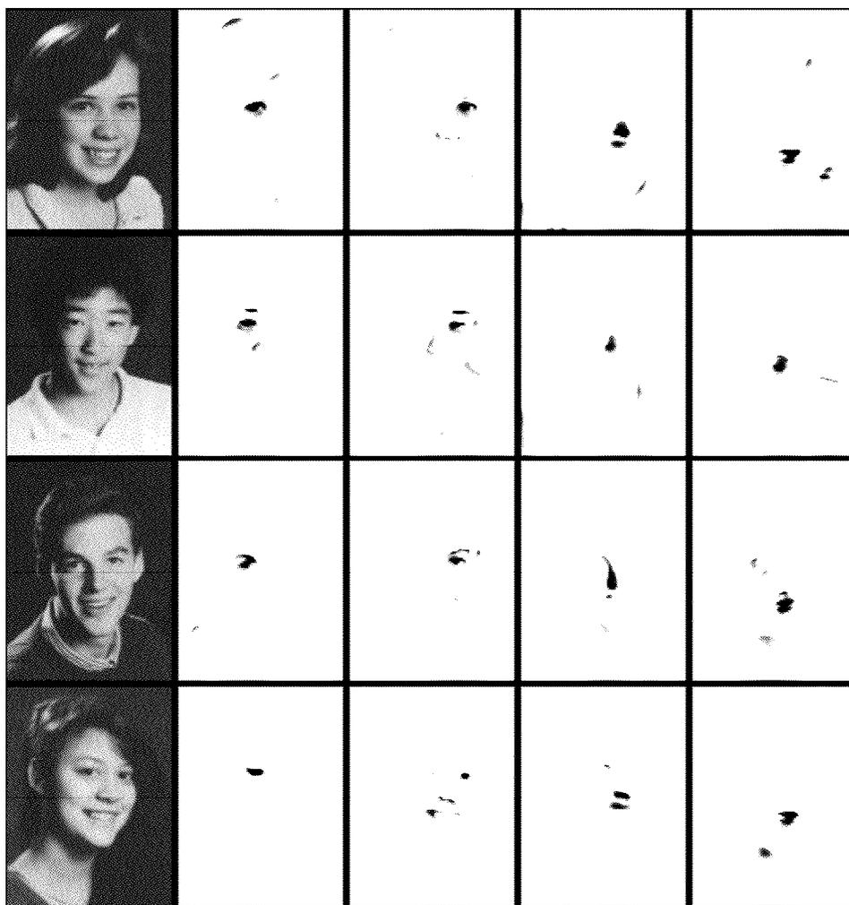
The four images in the testing set and the neural network's corresponding feature maps, shown to the right of each image. Their order, from left to right, is left eye, right eye, nose, and mouth. "Left eye" actually refers to the person's right eye, which appears closer to the left of the image.
