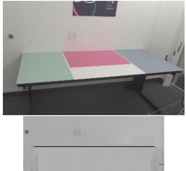
Figure 11: The top image shows a part of a wall that becomes noticeably colored from light reflecting from the cards placed on the table below, an effect known as "color bleeding". The bottom image shows the recovered albedo map of the same part of the wall. It is nearly uniform, showing that the color bleeding was properly accounted for. The black line has been added to indicate where the table top abutted the wall.
