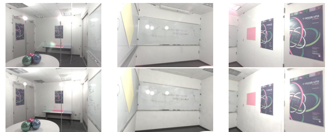
Figure 12: A comparison between real images (top) and synthetic renderings of our room with the recovered reflectance parameters (bottom). The simulated lighting is the same as in the original pictures, and the synthetic viewpoints have been matched to the recovered camera positions of the real images. The images show that good consistency was achieved.
