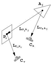
Figure 3: Patch  $A_j$  is in the radiance image captured by camera  $C_k$ . The specular component at  $A_j$  in the direction of sample point  $P_i$  is different from that in the direction of camera  $C_k$ . The difference is denoted by  $\Delta S$ .
