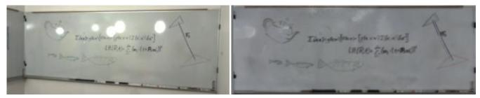
Figure 10: The left picture is a radiance image of a whiteboard, showing strong specular highlights. The right picture shows the diffuse albedo map of the whiteboard recovered from several images. Unlike the radiance image, the diffuse albedo map has a nearly uniform background, and is independent of the illumination.
